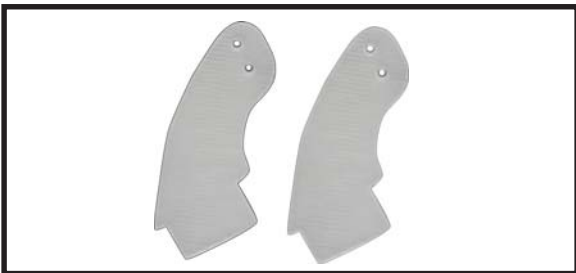
Control horn of Rudder.
